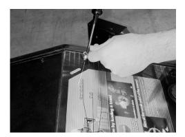
Lift the Control Panel to reveal the Star Button Lamp Housings. Hold the housing and gently pull to disengage the lamp housing from the button. The Bulb is a "push to fit" bulb and is removed by pulling the bulb from within the housing.
