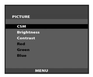
Use the UP and DOWN Buttons to move the 'Black Bar'to the item you want to adjust. After selecting the desired item, pressing the SELECT Button will extend the MENU Screen and allow adjustments to be changed.
